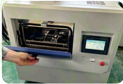
Solar Radiation & Temperature & Humidity aging equipment
